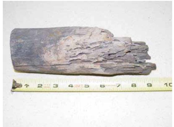
**Wooden plug that was blown out of a well in West Point.**
